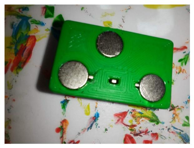
Don't forget to install the magnet which holds the probe to the probe dock.
