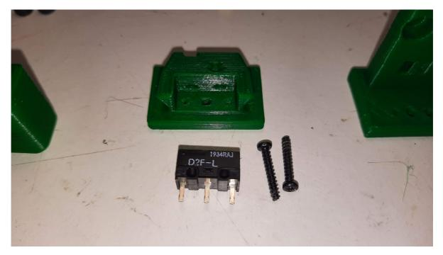
Maybe you need to clear the holes for the microswitch, a 1.5mm drill bit should work fine.
