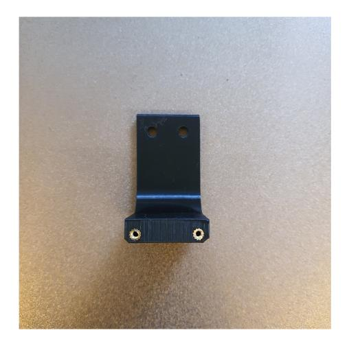
Install the magnet in the Probe dock and screw it onto the Dock mount with the two M3x20mm SHC screws.
