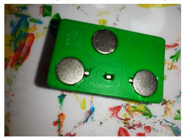
Don't forget to install the magnet which holds the probe to the probe dock.
