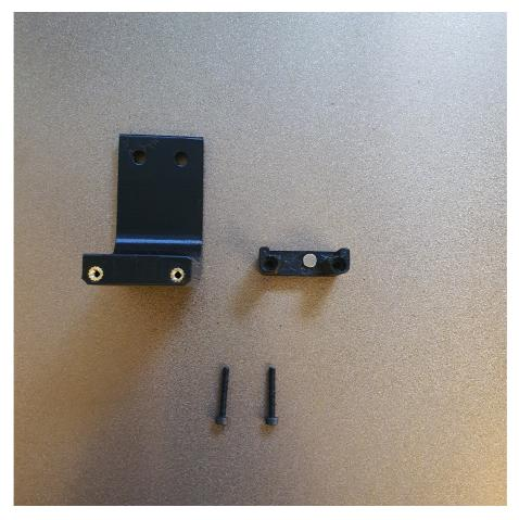
Mount the Probe Dock to the back rail of your gantry with the two M5x10 and the two roll in nuts.
