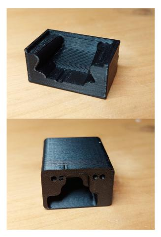
Insert the AB mount and probe in the helper parts and you can then press fit with a vice or on a hard surface.
