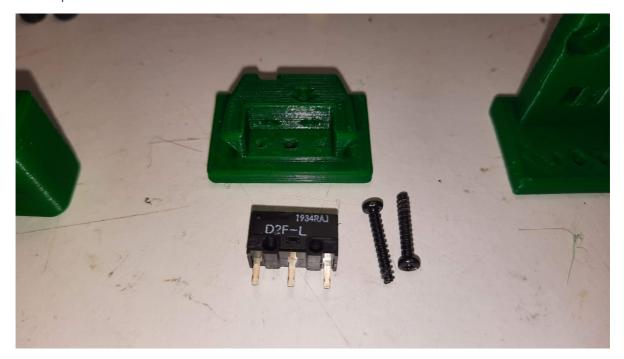
Maybe you need to clear the holes for the microswitch, a 1.5mm drill bit should work fine. Install the microswitch so that the arrow on the probe body is pointing to the little switch.
