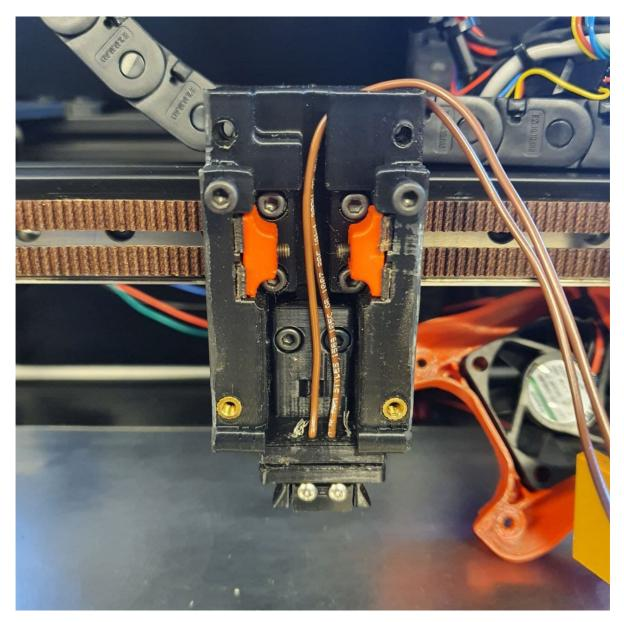
Connect the two wires from the Klicky Probe to the GND and Signal of the recommended Probe signal for your board, you can even leave the BAT85 that is necessary for the 24v inductive probes.
